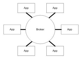
**Solution:** Use a central message broker that can receive messages from multiple destinations, determine the correct destination and route the message to the correct channel. The message broker pattern is also known as a hub-and-spoke architecture.
